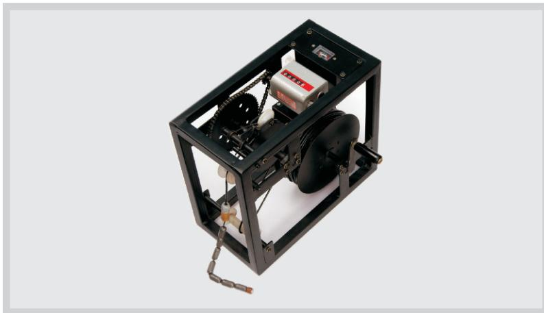
**IGIS has introduced new Water Level indicator with counter mechanism is a very handy device to quickly check the level of water in open wells and in borewells.**
